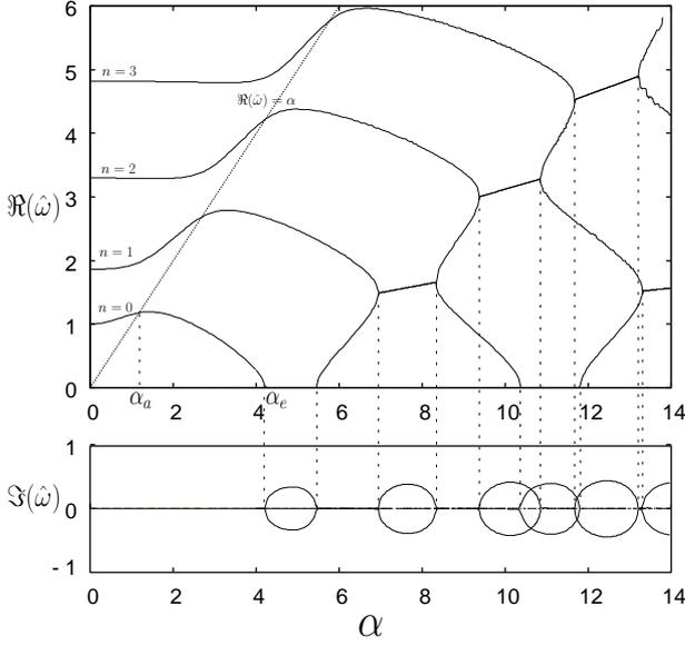
Figure 4: Eigenvalue diagram  $\hat{\omega}_n - \alpha$  of acoustic modes for fixed  $k = 1$ . The right hand side of the dashed line  $\Re(\hat{\omega}) = \alpha$  is filled with the continuous spectrum  $\sigma_c = [-\alpha, \alpha]$ .
